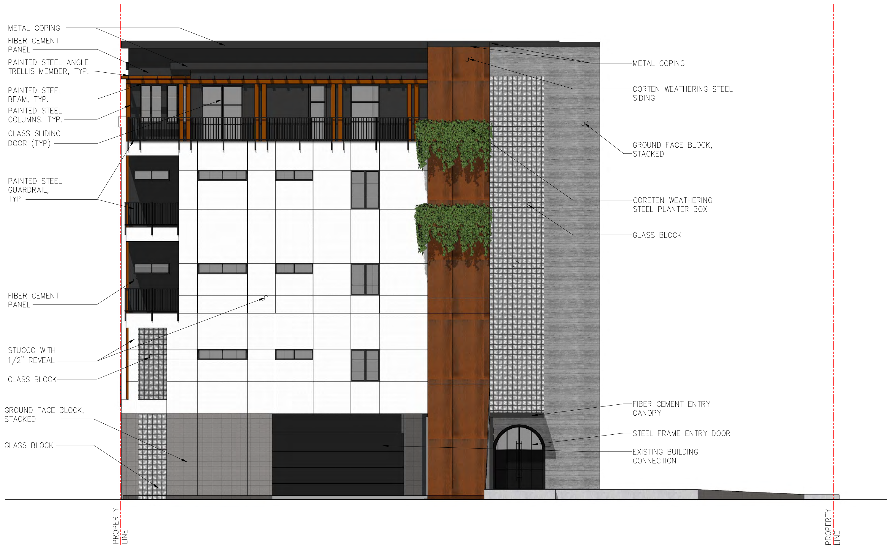
2 EAST EXTERIOR ELEVATION 1/8"=1'-0"
