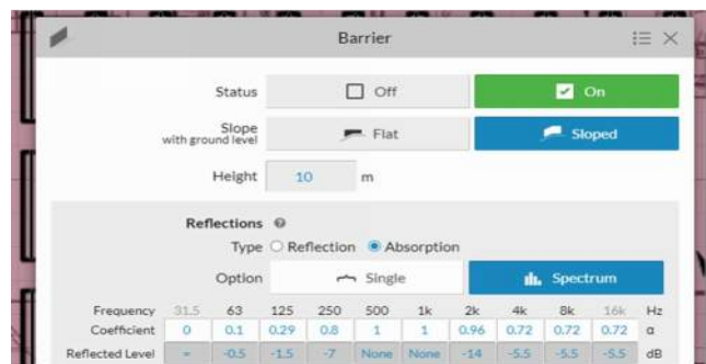
Figure 5. Acoustic Barrier Properties
