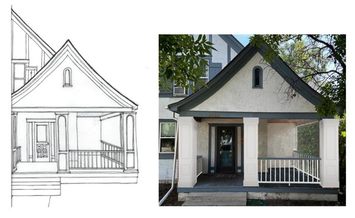
The exterior finishes are white columns matching the body color of the home, the top of the handrail assembly is blue to match the trim color and the bottom rail is white. Again, to match the body color of the home. The balusters or vertical picket are square (1  $\frac{1}{2}$ ") and white in color to match the house.
