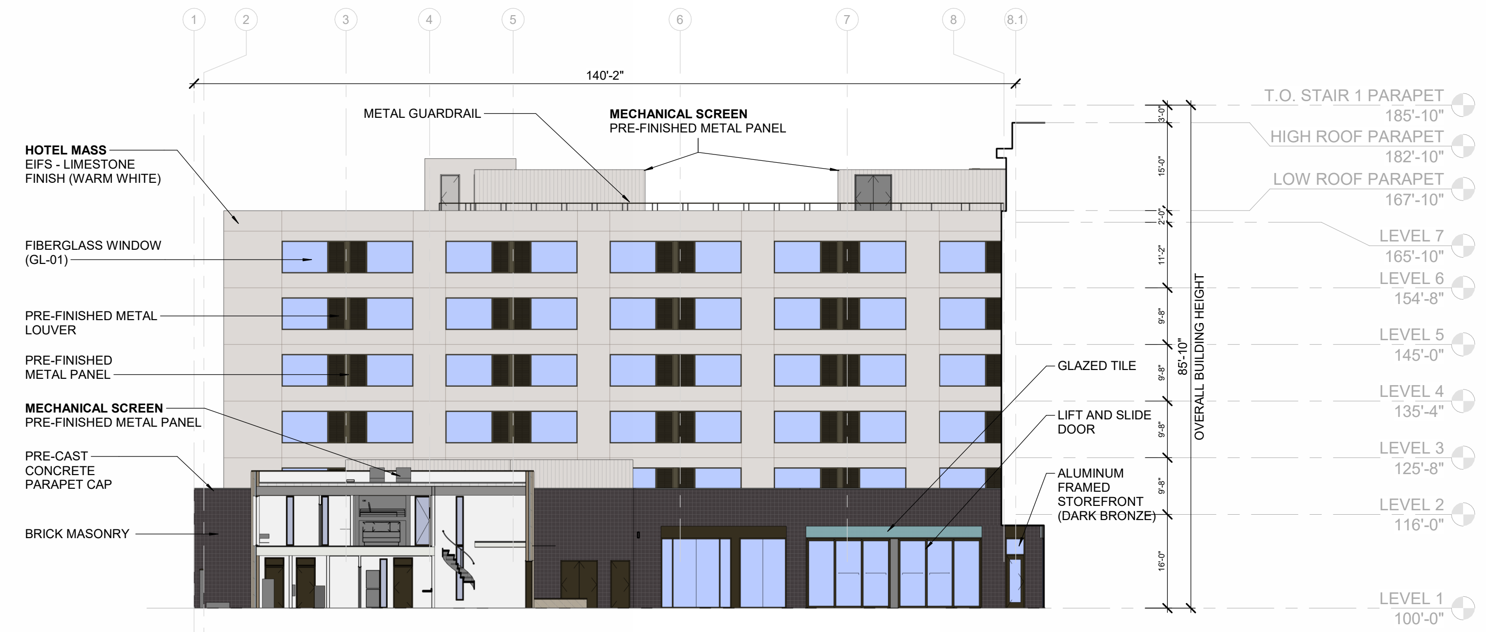
1 INTERNAL NORTH ELEVATION 1/16" = 1'-0"
