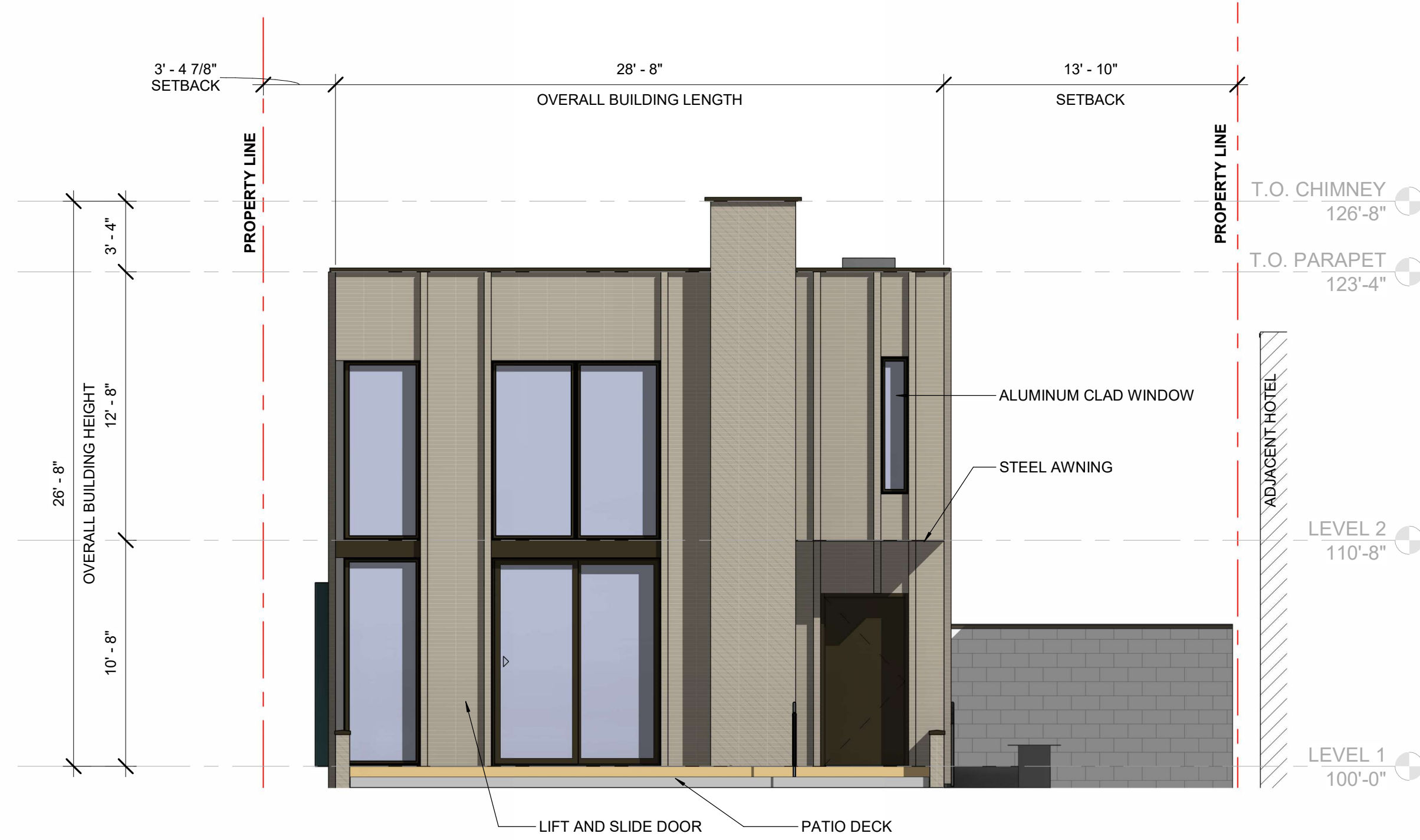
4 KLEE HOUSE - EAST ELEVATION 3/16" = 1'-0"
