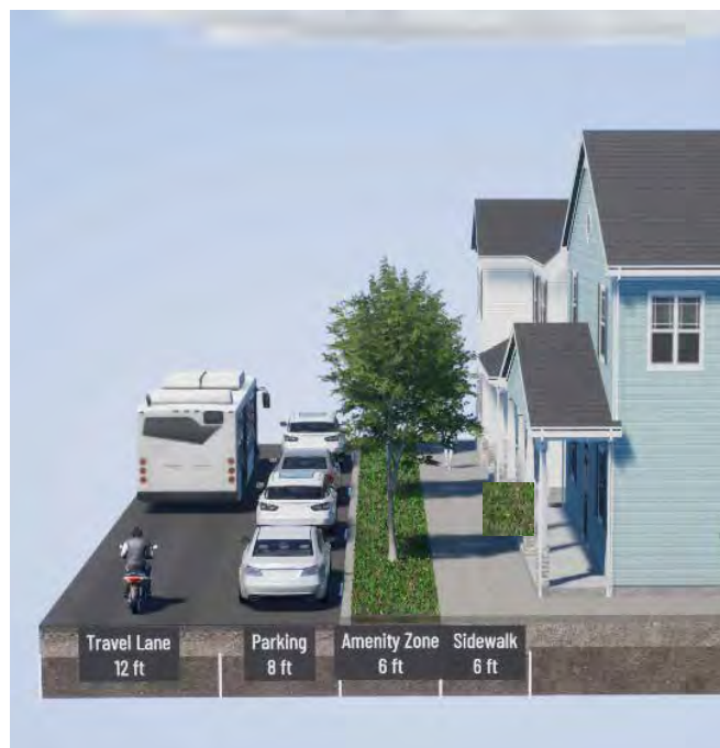
Figure 4.16 | Cross-section depicting a detached sidewalk six feet in width, the preferred configuration
