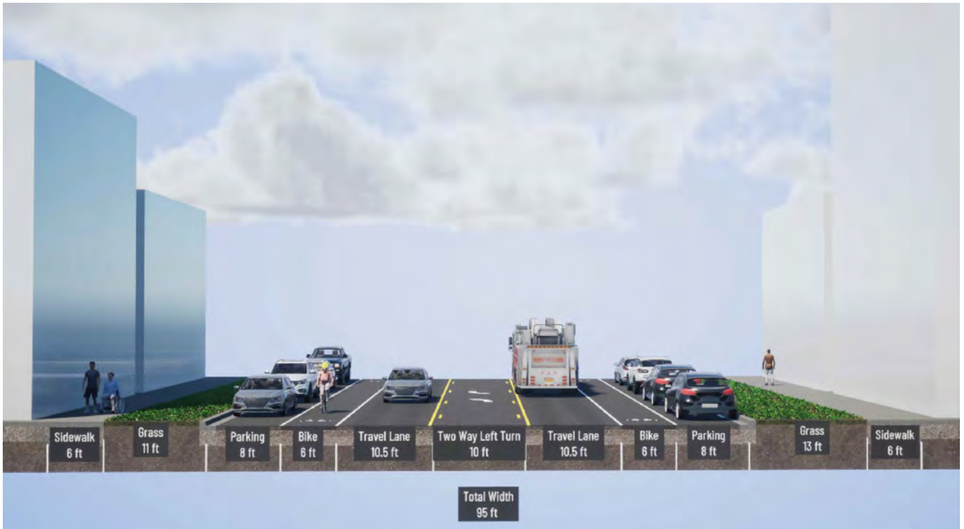
Figure 4.14 | Existing: Typical Active Transportation Priority Street Example
