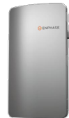
IQ System Controller 3/3G Provides microgrid interconnection device (MID) functionality by automatically detecting grid failures and seamlessly transitioning the home energy system from grid power to backup power.
