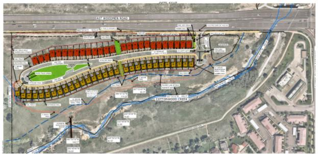
**Access:** Access to the property will be from East Woodmen Road via a 3/4-movement access to allow a left-in turn for westbound traffic on Woodmen Road. A new sidewalk will be constructed with the development along Woodmen Road, which will also provide connectivity to the Cottonwood Creek Trail, Briargate Trail, and Woodmen Trail east of Austin Bluffs Parkway.
