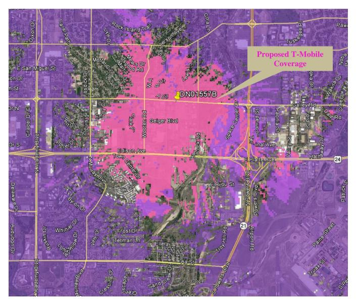
There is improvement in coverage and service quality around the proposed site and in all areas listed above. We have continuous quality coverage between existing sites north and south. The site fills the residential gap in coverage and improves existing site capacity offload. We are meeting most of our objectives.
