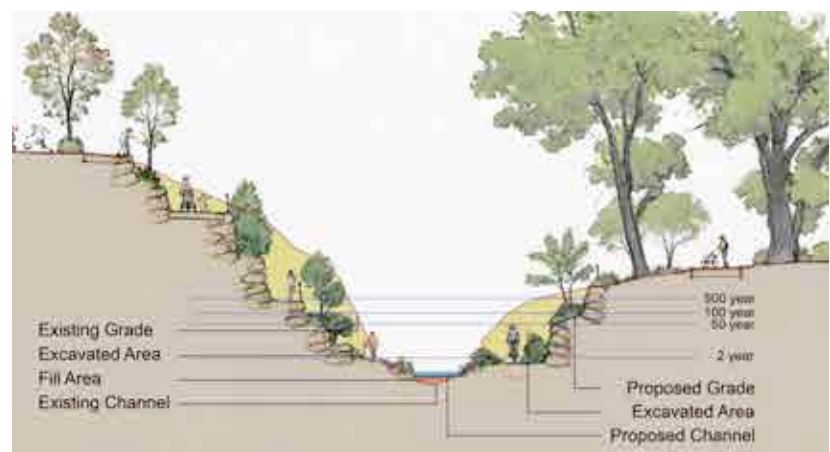
Figure 25: Asymmetrical Channel Banks
