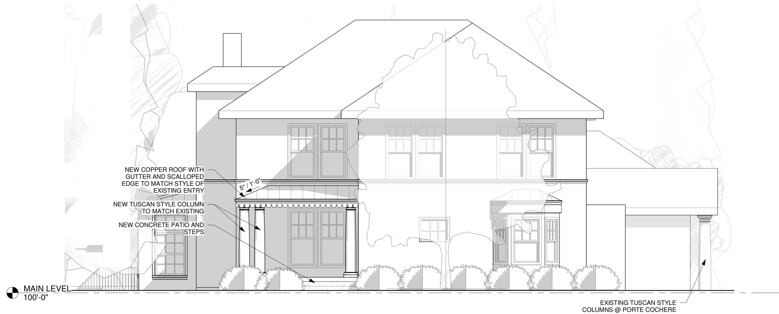
2 EXTERIOR ELEVATION - FRONT (EAST) - COVERED ENTRY 3/16" = 1'-0"
