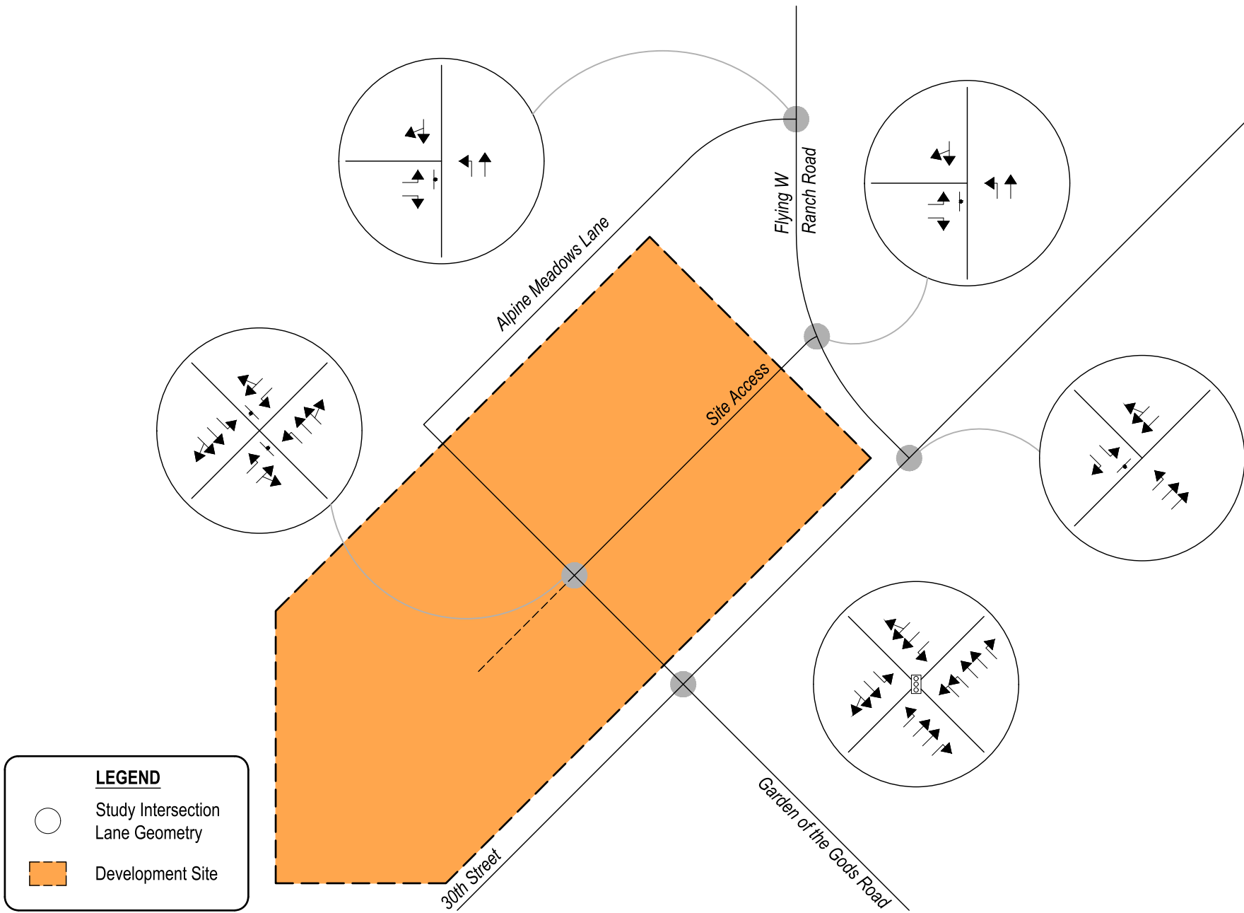
Figure 8a TOTAL TRAFFIC - YEAR 2042 Intersection Geometry
