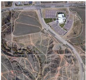
Site soils are primarily sandy loam. The three types of soil are Chaseville-Midway Complex, Ascalon sandy loam (3-9% slopes) and Razor-Midway complex. The main limitations for construction are slope. The geology study notes that Pierre Shale (Kp) is easily excavated but foundation stability is poor. Colluvium (Qc) areas are susceptible to future colluvial deposition mudflows, and landslides. Older gravel 2 (Qg2) is a well-developed pedogenic soil and is suitable for development.
