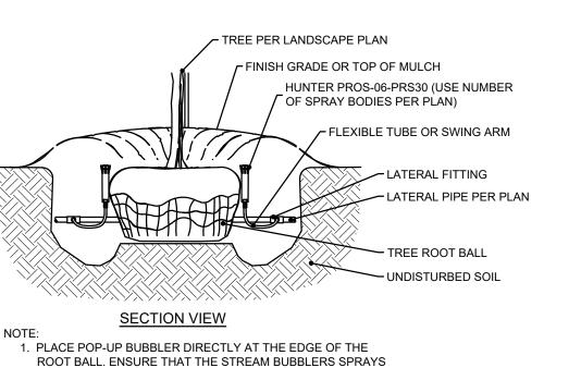
2. SPACE REQUIRED NUMBER OF SPRAY BODIES EQUIDISTANT AROUND EDGE OF ROOT BALL. 2. USE NUMBER OF SPRAY BODIES PER PLAN. **│ TREE BUBBLER ASSEMBLY WITH HUNTER PROS-06-PRS30**
