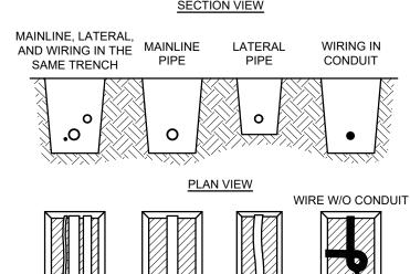
TIF A 24-INCH LOOP IN ALL WIRING RUN WIRING BENEATH ALL SOLVENT WELD -AND BESIDE MAINLINE. PLASTIC PIPING TO AT CHANGES OF DIRECTION OF 30° TAPE AND BUNDLE AT BE SNAKED IN OR GREATER. UNTIE AFTER ALL 10-FOOT INTERVALS. TRENCH AS SHOWN. CONNECTIONS HAVE BEEN MADE.
