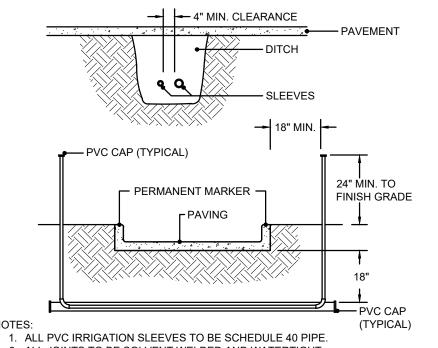
2. ALL JOINTS TO BE SOLVENT WELDED AND WATERTIGHT
