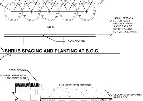
RIVER ROCK TO BE COMPACTED TO A 3" DEPTH **DECOMPOSED GRANITE / RIVER ROCK**
