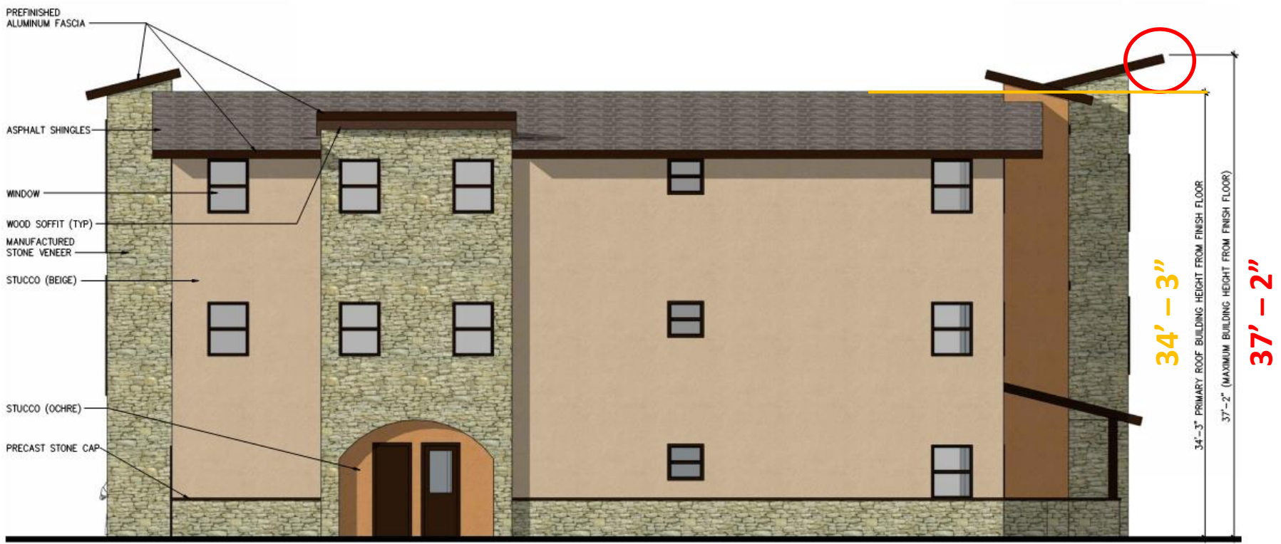
4 TYPICAL SIDE ELEVATION (UNLESS NOTED OTHERWISE) 3/16" = 1'-0"
