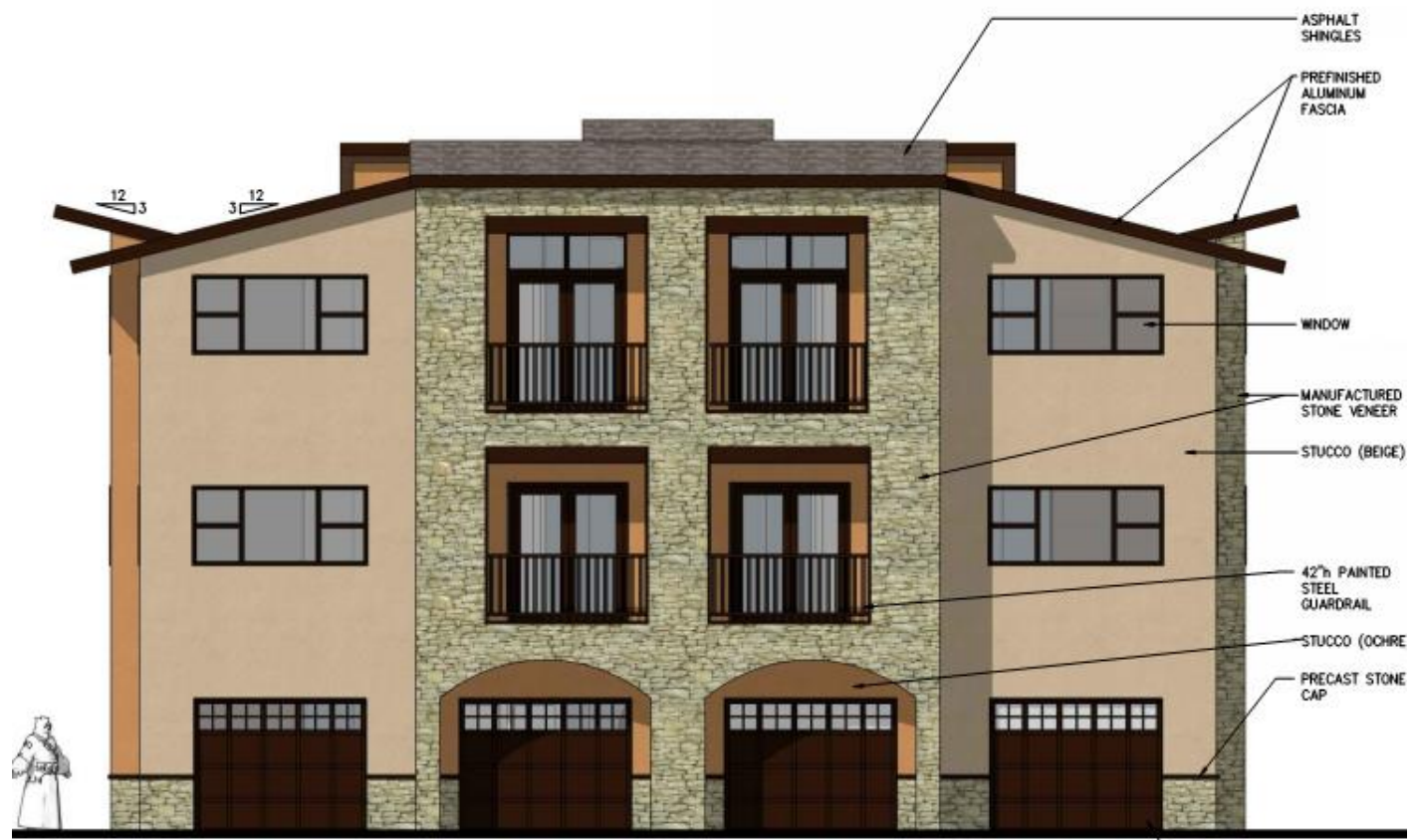
2 TYPICAL EAST ELEVATION 3/16" = 1'-0"
