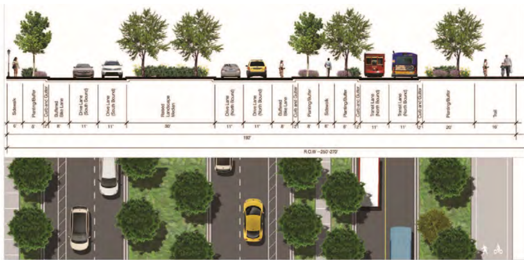
Proposed Nevada Avenue Typical Section with dedicated multi-modal corridor
