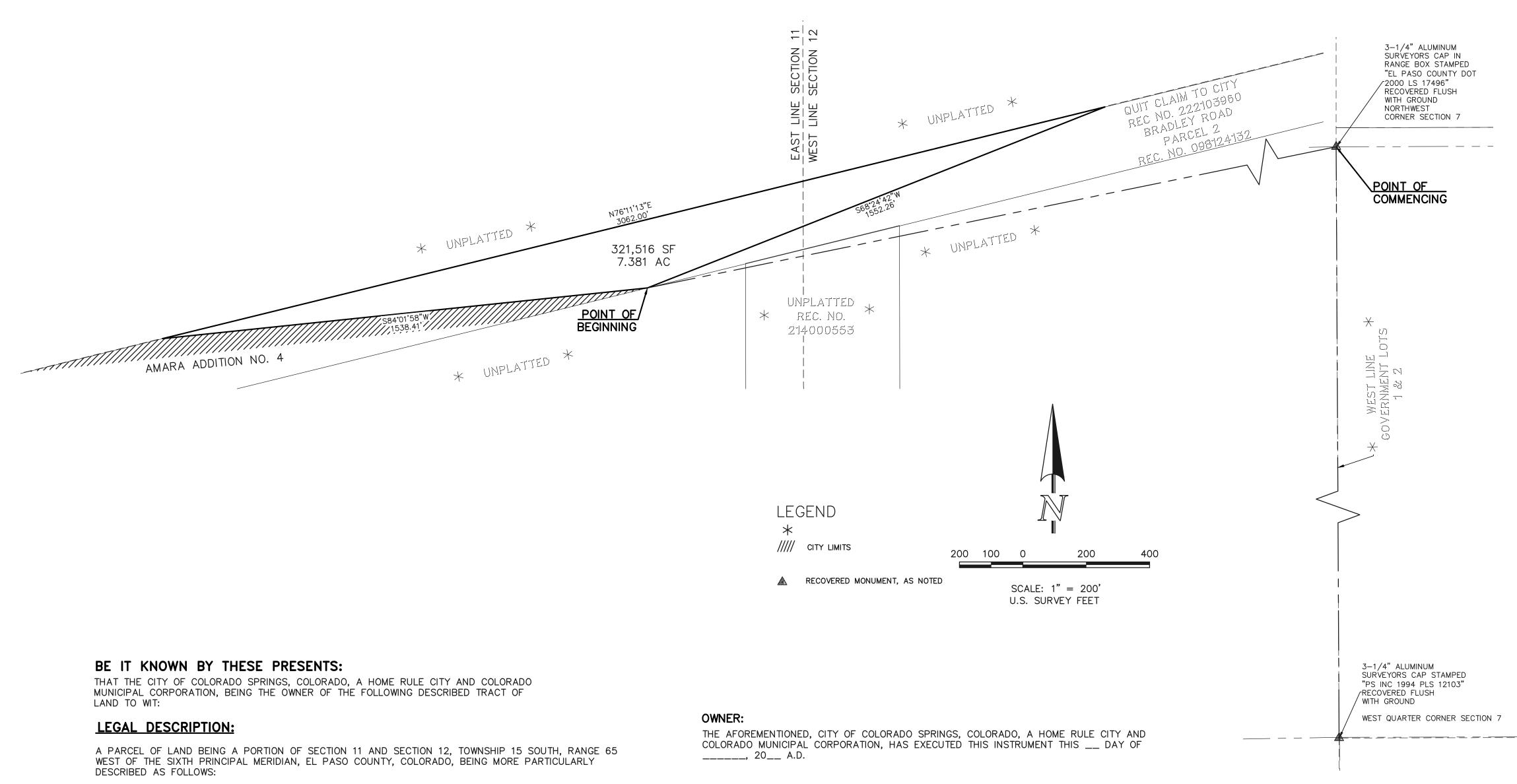
BASIS OF BEARINGS: THE WEST LINE OF GOVERNMENT LOTS 1 AND 2, IN SECTION 7, TOWNSHIP 15 SOUTH, RANGE 64 WEST OF THE SIXTH PRINCIPAL MERIDIAN, BEING MONUMENTED AT THE NORTHERLY END BY A 3-1/4" ALUMINUM SURVEYORS CAP IN RANGE BOX STAMPED "EL PASO COUNTY DOT 2000 LS 17496: FLUSH WITH GROUND AND AT THE SOUTHERLY END BY A 3-1/4" ALUMINUM SURVEYORS CAP STAMPED "PS INC 1994 PLS 12103" FLUSH WITH GROUND IS ASSUMED TO BEARS NOO'17'10"W, A DISTANCE OF 2635.08 FEET.
