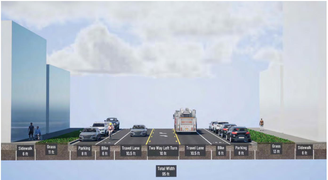
Figure 4.14 | Existing: Typical Active Transportation Priority Street Example
