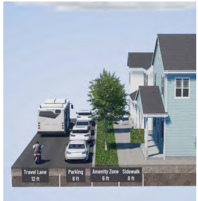
Figure 4.16 | Cross-section depicting a detached sidewalk six feet in width, the preferred configuration
