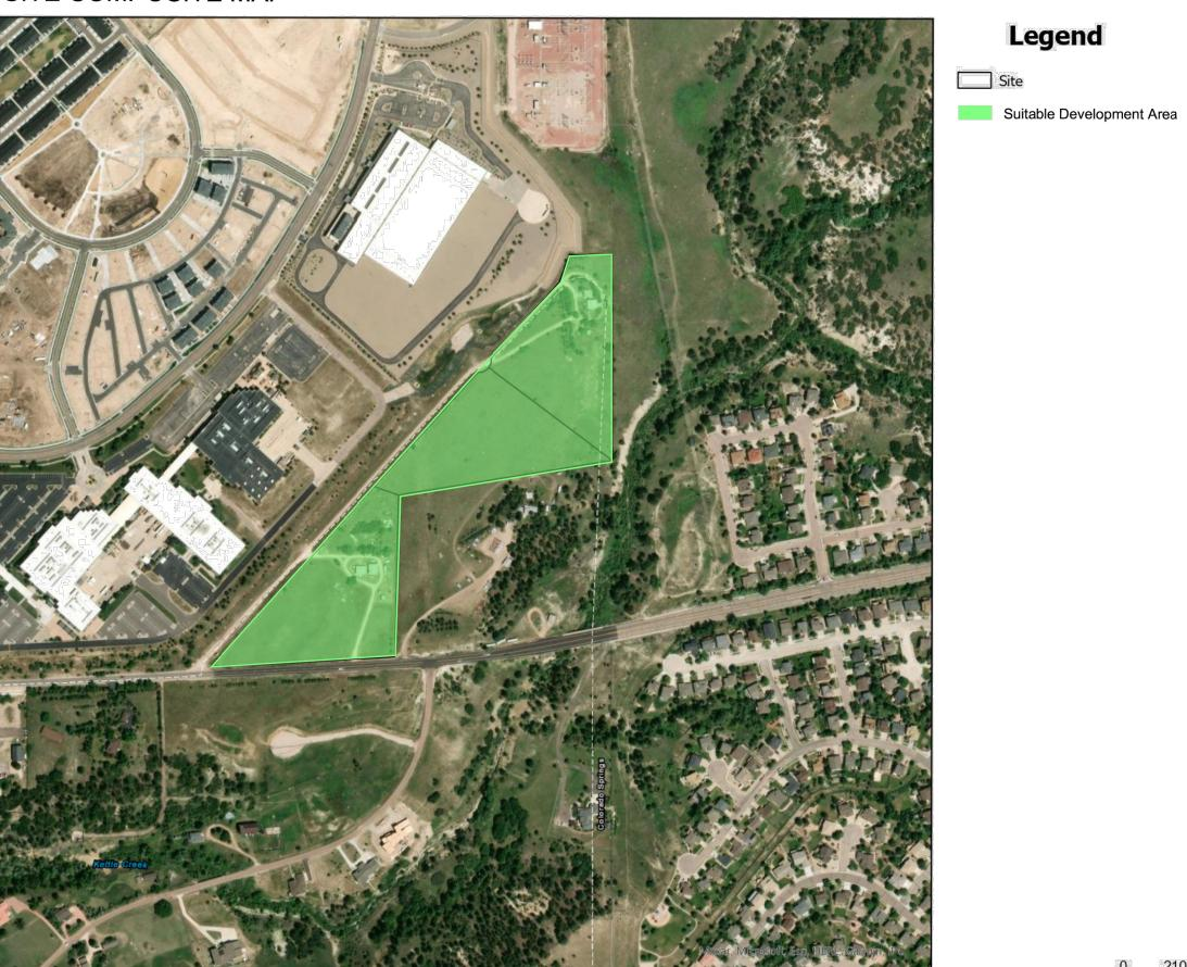
THE COMPOSITE MAP CONCLUSION IS THAT THE SITE IS BUILDABLE. AFTER ANALYSIS OF THE SOIL, TOPOGRAPHY, VEGETATION, GEOLOGY, HYDROLOGY, AND EXISTING CONDITIONS IT IS DEEMED TO BE SUITABLE FOR DEVELOPMENT. THE DEVELOPMENT SHOULD STAY CLEAR OF THE STREAMS AND REQUIRES MEASURES TO PROTECT WATER QUALITY. TREE PRESERVATION SHOULD TAKE PLACE WHEN POSSIBLE.
