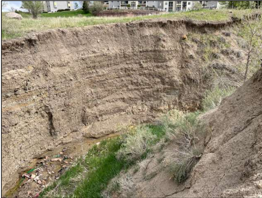
11. Facing southeast across a typical section of the eroded gully/Open Water F. Dark clay soils with orange oxidization were observed along the walls of the gully from top to bottom. May 21, 2021.
