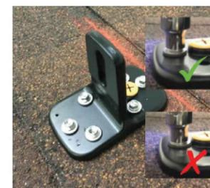
**ATTACHING TO A RAFTER:** Place FLASHLOC DUO over rafter location and align upper edge of mount with horizontal chalk line. Secure mount with the two (2) provided rafter screws. **BACKFILL ALL PILOT HOLES WITH SEALANT.**
