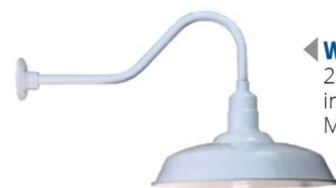
W520-42WPL-RTC-E6-200GLFR-GUP-44 20" Warehouse Shade with Frosted Glass, Wire Guard, E6 Arm in White and RTC Ballast Housing with Fluorescent Ballast. Fluorescent ballast accommodates 26WCFL, 32WCFL, or 42WCFL. Also available in Clear Glass.
