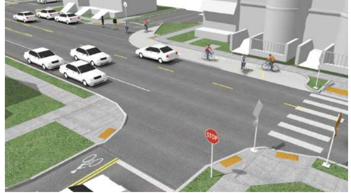
Offset intersection treatment using two-way separated bike lane (from NACTO)
