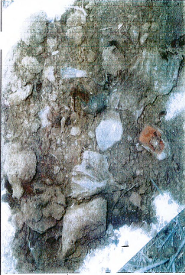
Photograph 14 - Looking at small pieces of glass, wood, and plastic that was collected in Boring S2-2.
