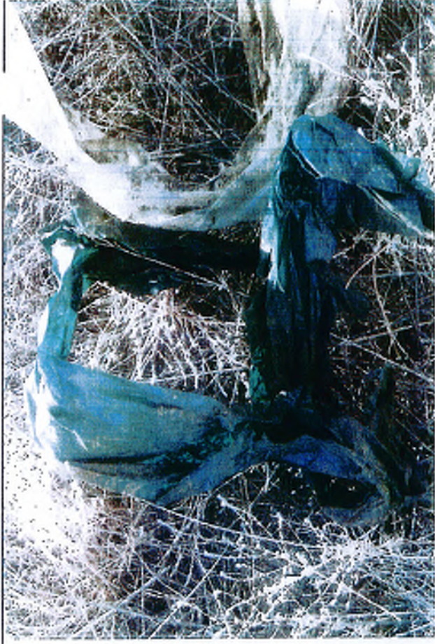
Photograph 18 - Looking at large amounts of plastic that were pulled out of Boring S2-3 during drilling.
